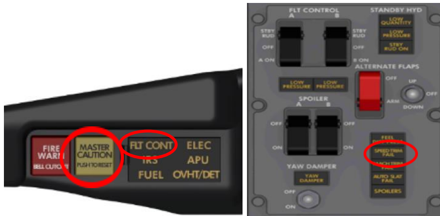
FIGURE 2 SPEED TRIM FAIL ANNUNCIATION
