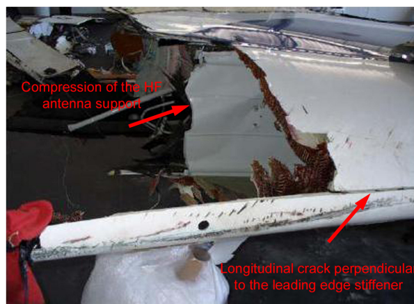
Figure 46: HF antenna support
