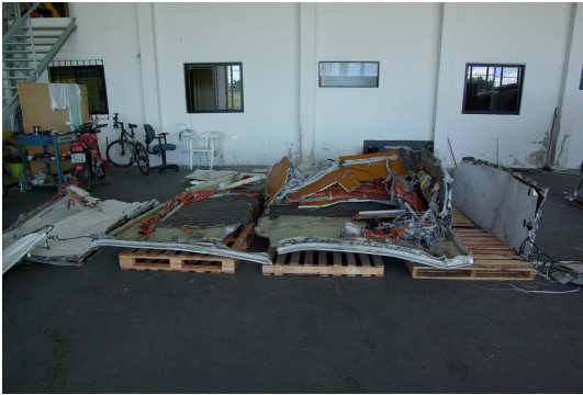
Figure 38: Floor of the LDMCR: with bottom-upwards deformation
