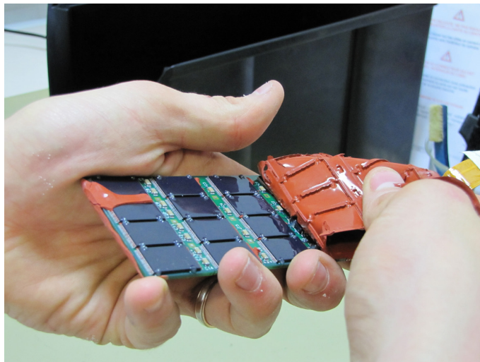
Figure 20: Removal of internal protective layers
