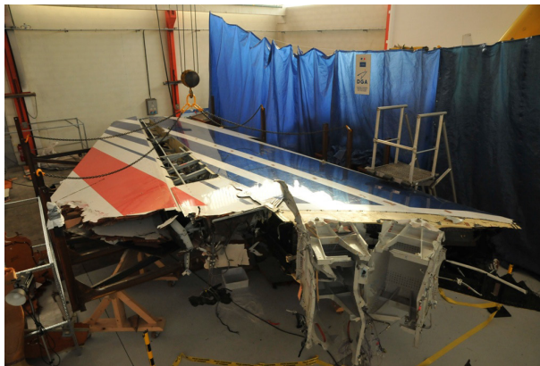
Figure 44: Fin – In the foreground the base of the fin with the central and forward attachment lugs
