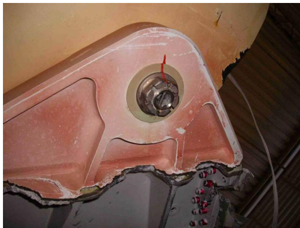
Figure 49: Right-hand aft lug: shearing of the fuselage along main frames 86-87
