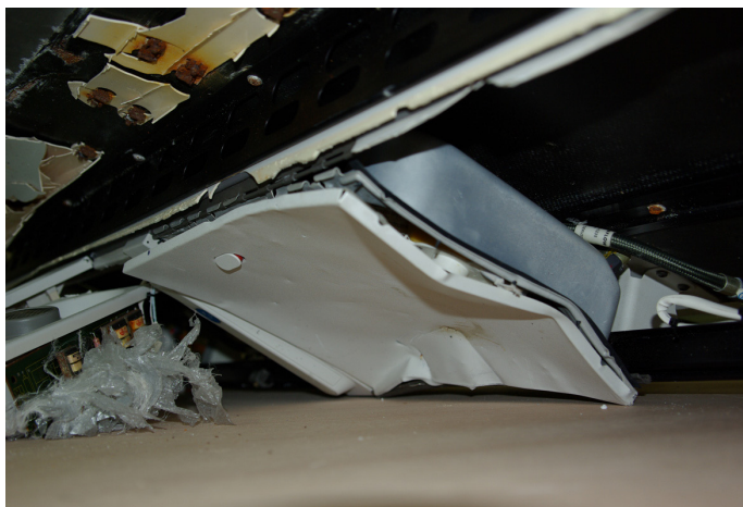
Figure 40: Passenger oxygen container recovered closed: the deformations on the cover matched those on the box
