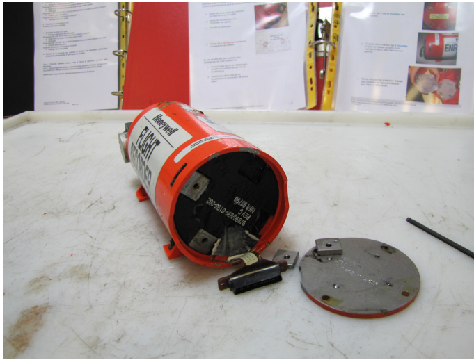
Figure 21: Opening of CVR CSMU
